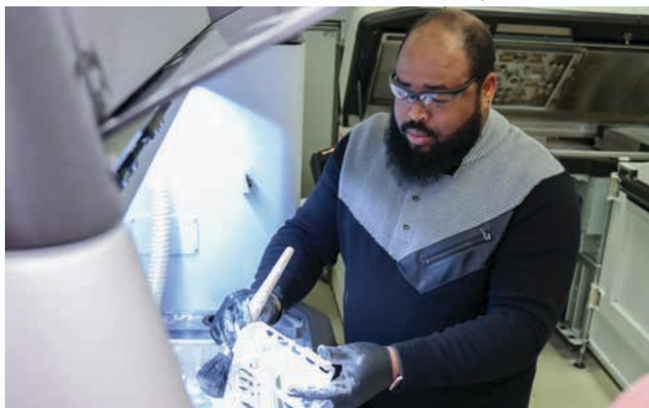
DEVCOM CBC Engineering Technician, Rashad Scott, brushes away powder to reveal a plastic part created through a type of advanced manufacturing called multi-jet fusion, or MJF.
