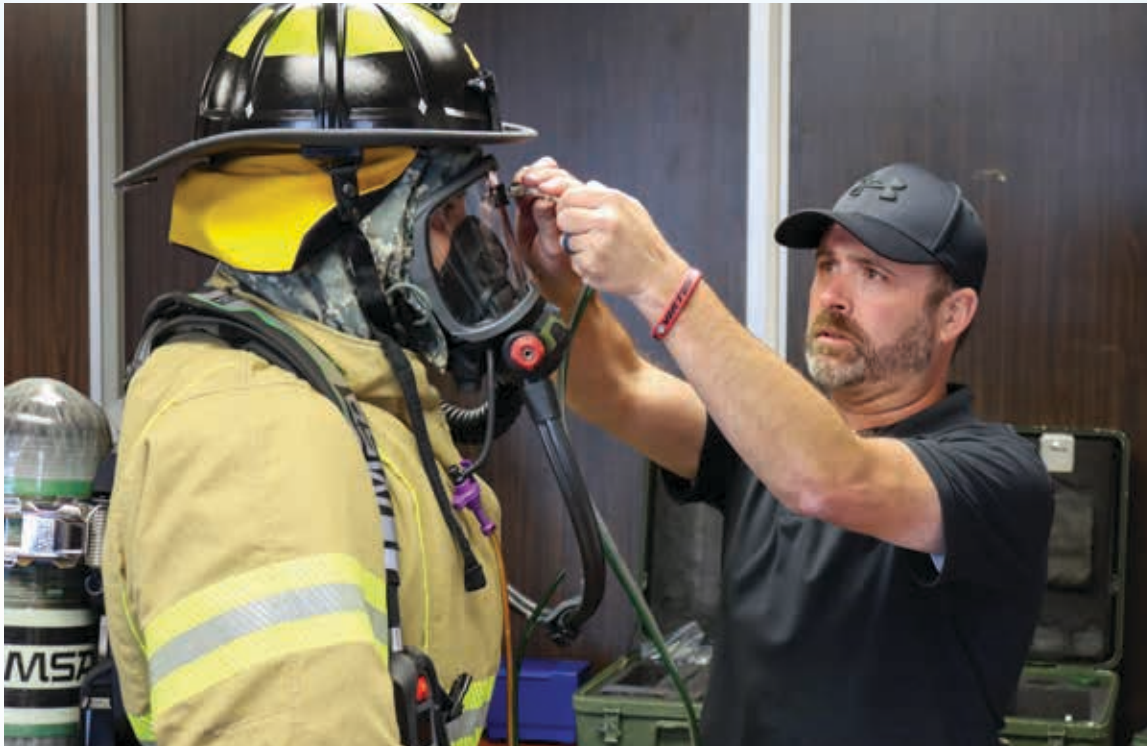
DEVCOM CBC Lead Engineering Technician, Justin Geldof, attaches a tube to a prototype gasmask to test its airtight seal.
