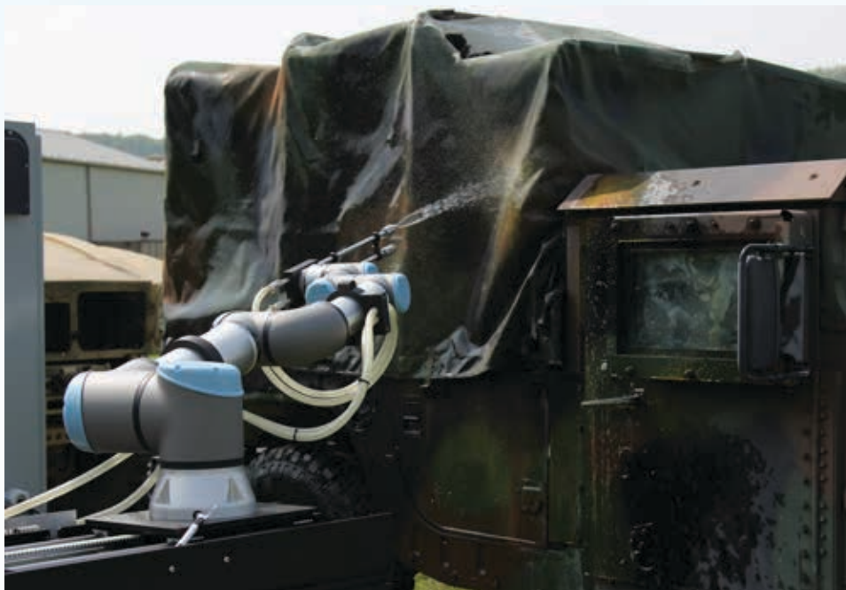
The Autonomous Equipment Decontamination System has been demonstrated at several exercises, including the Maneuver Support Protection Integration Experiments (MSPIX) at Fort Leonard Wood, Missouri in May 2024 and Chemical Biological Operational Analysis event held at Camp Dawson, West Virginia in August 2023 (shown in image).
