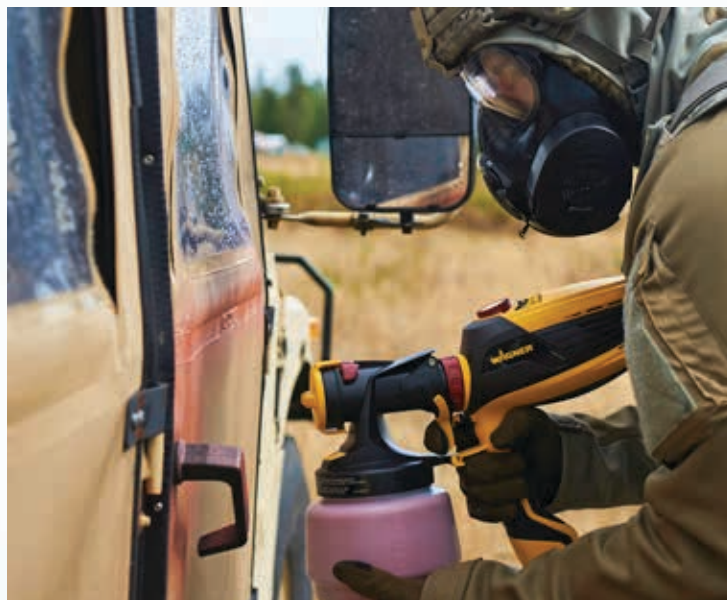
A soldier demonstrates the use of decontamination slurry, a paint-like substance that can decontaminate an entire vehicle with very little water.
