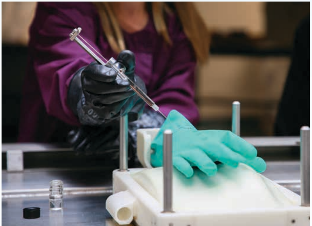
Jennifer Hughes, a DEVCOM CBC lab manager at Aberdeen Proving Ground Edgewood, Maryland, administers droplets of chemical testing agent on a glove to test its permeation capabilities for the Glove as a Glove initiative.
