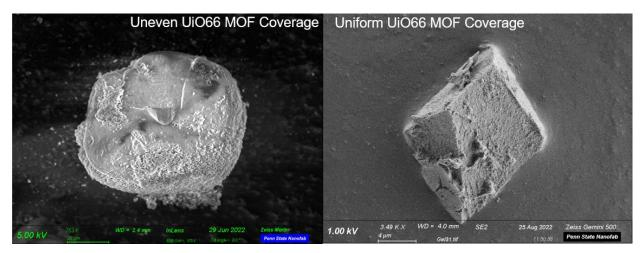
Figure 9. SEM images of UiO66@SiO2 Janus particles. The left image shows partial UiO66 coverage from Pennsylvania State University's first attempt without the proper reagents in stock. The right image shows complete UiO66 coverage from Pennsylvania State University's second attempt with the proper reagents in stock.
