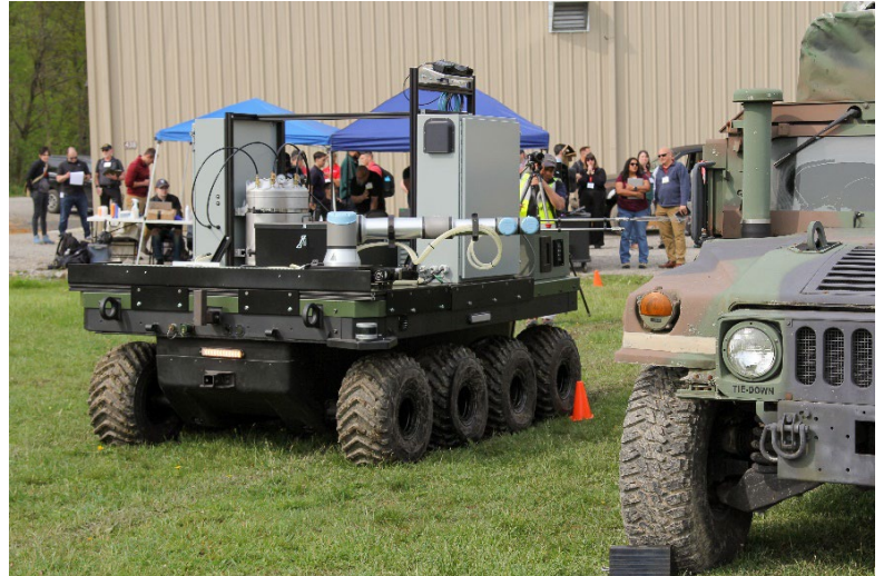
A UGV and custom-designed equipment controlled by remote operators decontaminates chemical agent simulant from a combat vehicle in a technology demonstration during CBOA 23 at Camp Dawson, West Virginia on May 11. (U.S. Army photo by Ellie White)
