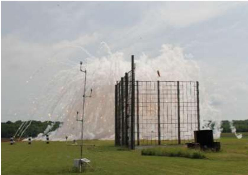
Vehicle-launched smoke grenades create an overhead smokescreen while various instruments gather data on the effectiveness of the smoke against visible and infrared observation. The DEVCOM CBC was part of a VIP demonstration held for Marine Corps officials seeking ways to protect vehicles from overhead attack.
