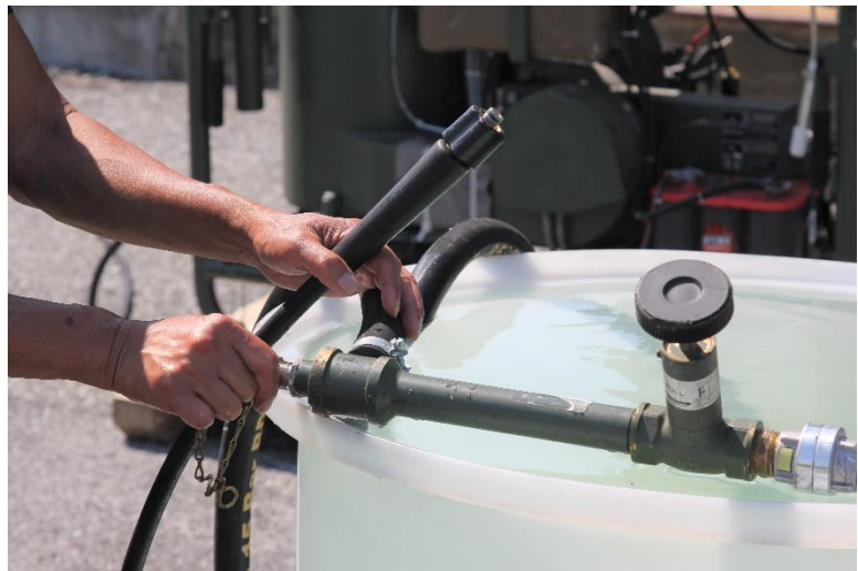
Kyle Hopkins, Maintenance Assistance and Instruction Team lead, connects spraying apparatus to the M26 decontamination system during the familiarization demonstration.
