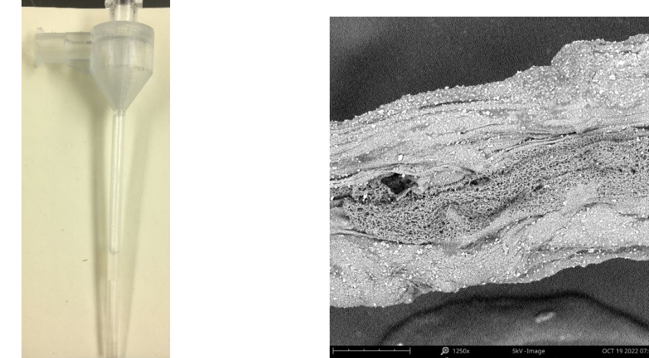
3D printed dual nozzle CMC-CS/MOF-808 wet spun Core-shell fiber
