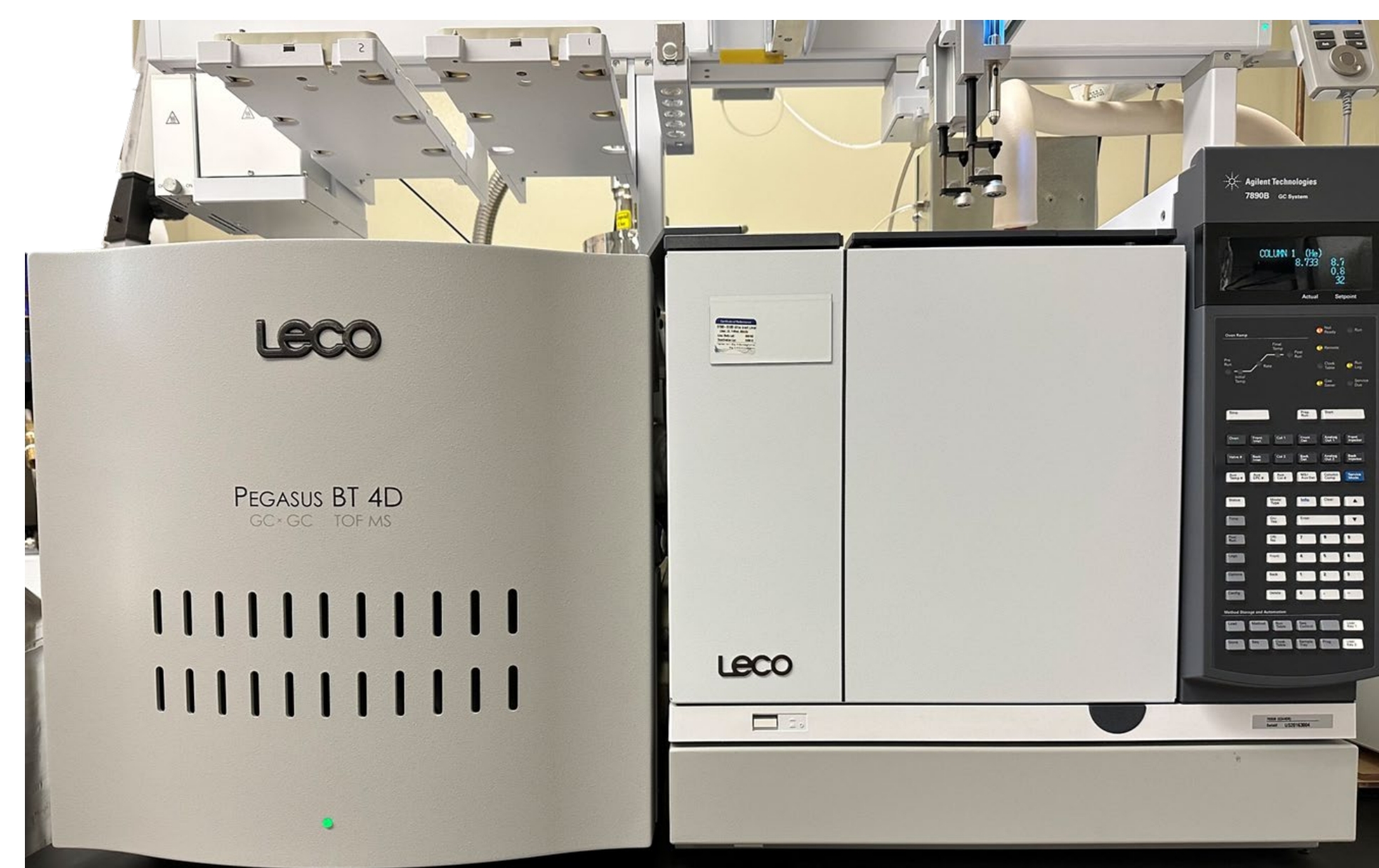
Figure 3: VOCs thermally desorbed onto LECO Pegasus BT 4D GCxGC TOF/MS
