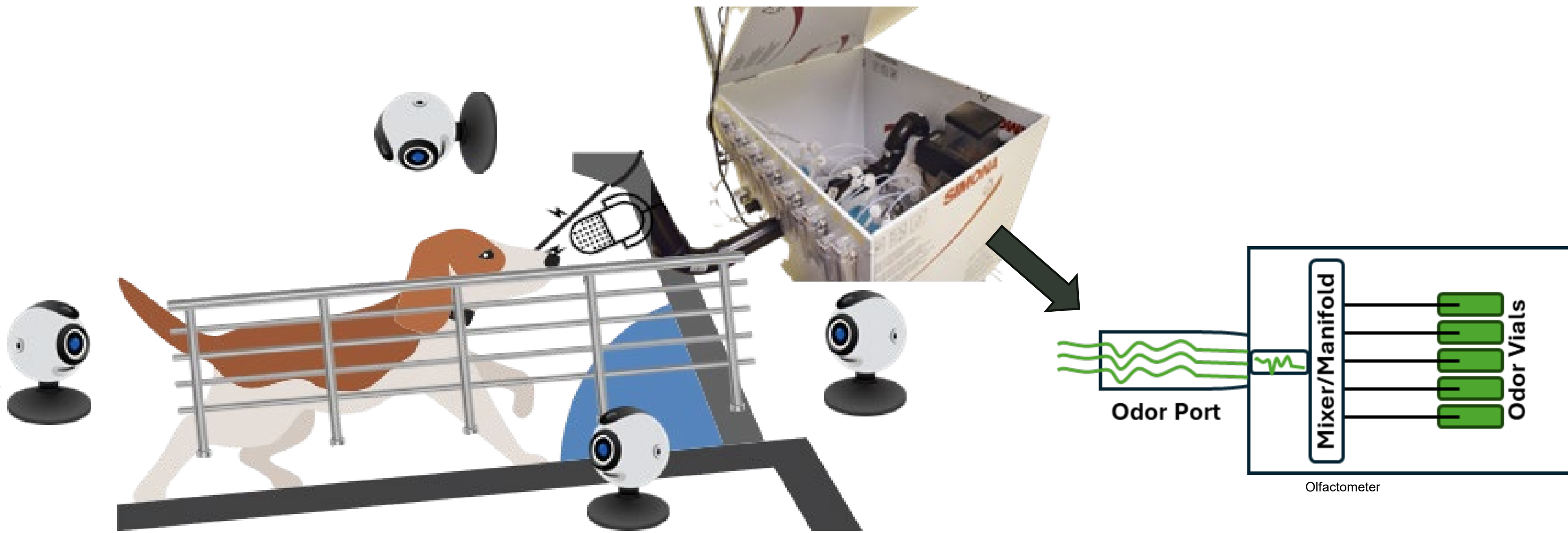
Figure 2. Canine Performance Assessment Treadmill Outfitted with cameras , microphones , and an olfactometer to assess canine olfactory performance via machine learning to predict behavior, endurance, and performance under physical stress. Arrow is indicating a schematic of the olfactometer mechanism on how odor is delivered to the dogs via the odor port.
