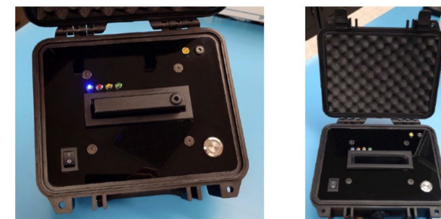
Figure 5. Automated Library Preparation Device. Automated library preparation prototype developed by Georgia Tech Research Institute (GTRI). The operator loads the purified DNA sample into a cartridge then places the cartridge into the slot and presses the start button. After the automated library preparation process is complete, the sample is removed and loaded onto the MinION sequencer.
