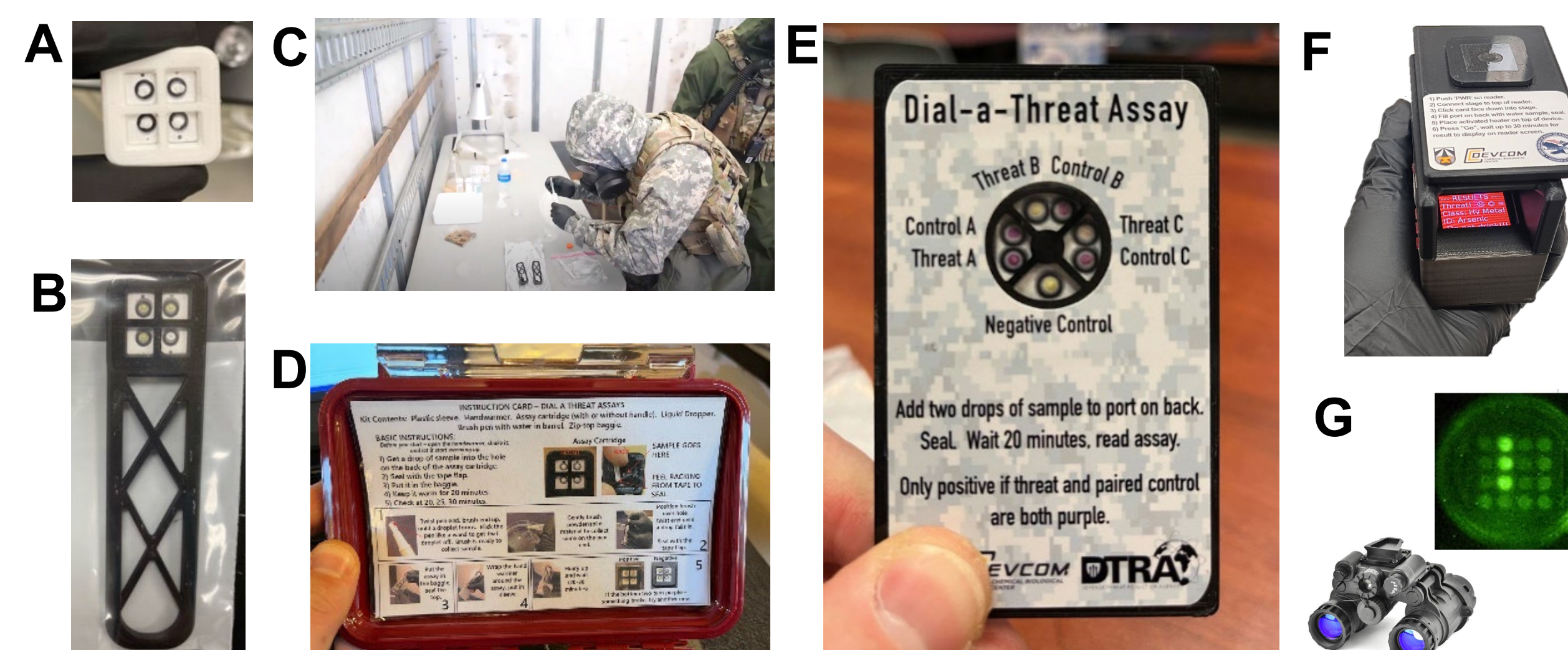
Figure 5: Field assessment and design progression. (A) Original design. (B) Design with handle to facilitate use with gloves. (C) Warfighter using Dial-a-Threat Device. (D) Pelican case with instruction set. (E) Dial-a-Threat card with 3-threat multiplexing and embedded instructions. (F) Portable reader for automated analysis and ATAK integration. (G) Night vision readout.
