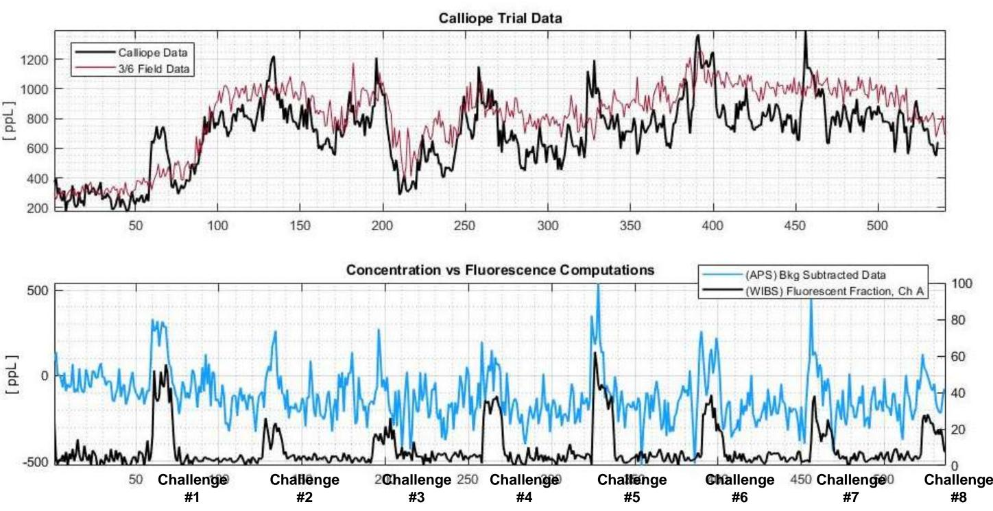
• A 4.5-hour test segment was selected from the field data. Calliope nozzles were then programmed to generate a test profile that matched the field segment to a 95% confidence interval as verified with variability and dynamics tolerance histogram reports.
