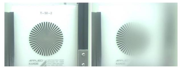
Photos taken at the start (left) and after 15 minutes (right) of a fogging trial conducted using a prototype respirator with no anti-fog coatings applied. Fog began creeping inward from the outside perimeter of the mask throughout the test, resulting in a half-fogged lens. The effects of the fog make the individual tines of the star chart indistinguishable on the right side of the right image.
