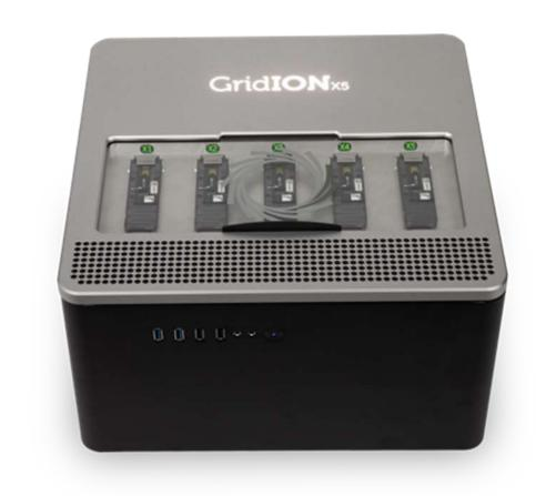
Nucleotides pass through the nanopore and produce a characteristic current change that is used to determine the corresponding nucleotide type at ~450 bases per second.
