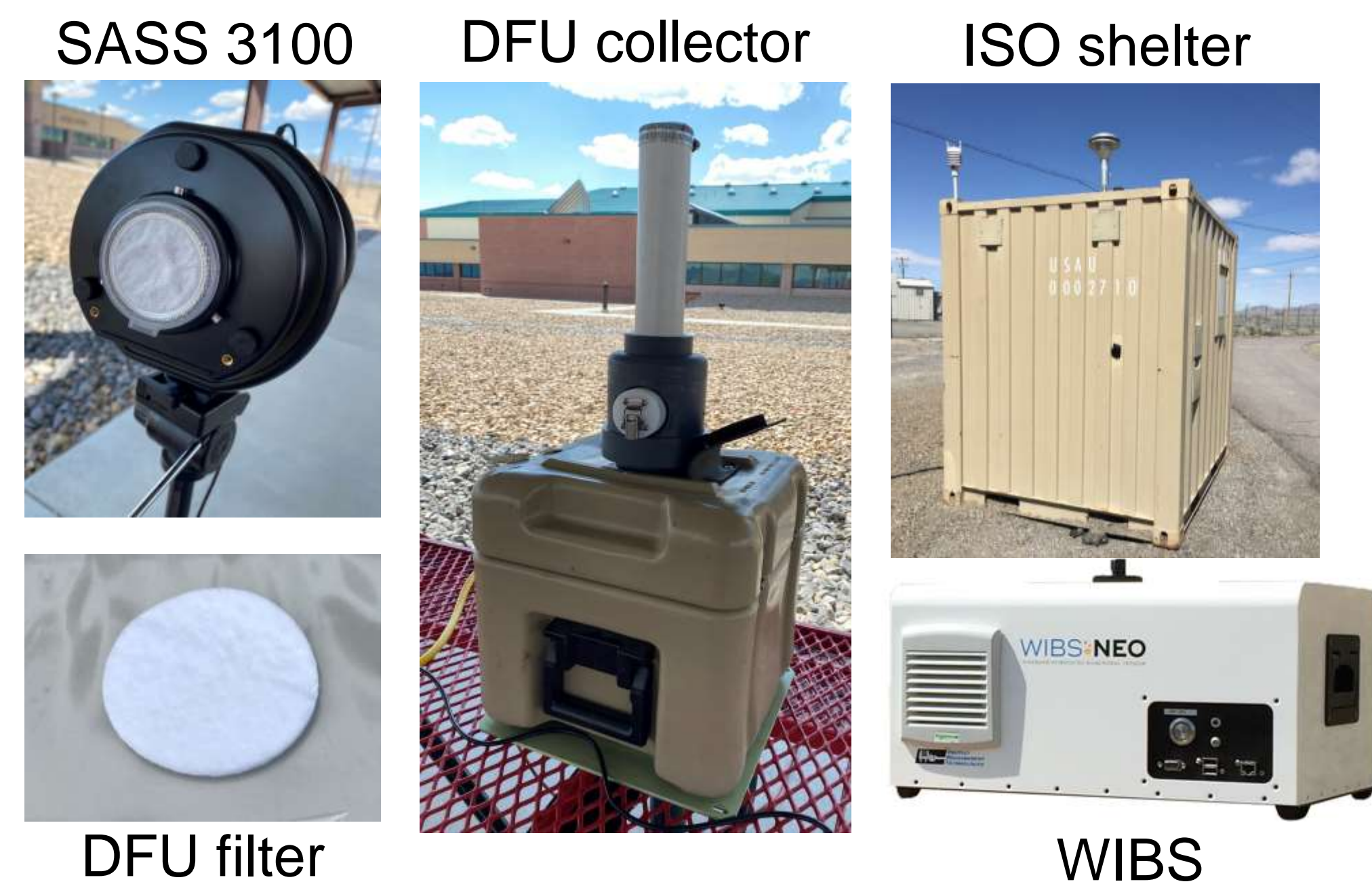
Figure 1. Sample collection and monitoring equipment for aerosol background study.
