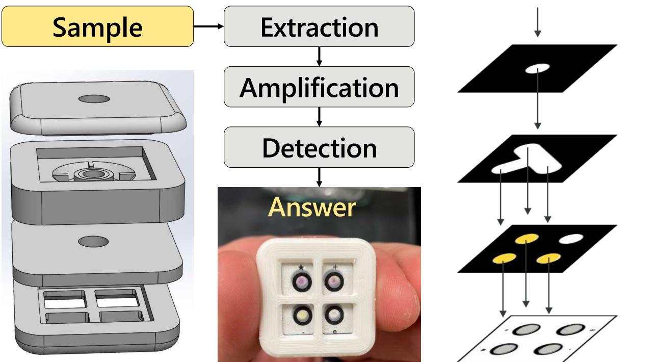
The "Dial a Threat" Assay: The design of our prototype is highly modular, with the main conserved element being high-performance lyophilized cell-free lysate. By swapping out modules the user can perform additional amplification reactions, and by putting different DNA sequences in the sample buffer, entirely different threat identification assays can be performed on the same device.
