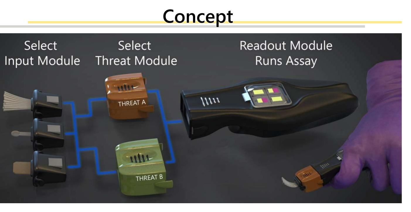
This project aims to integrate advancements in cell-free biology, synthetic biological detection circuits, 3D printing, and 'paperfluidics' to produce a means to perform next-generation biological (and eventually chemical) detection and identification in the field with minimal user burden.
