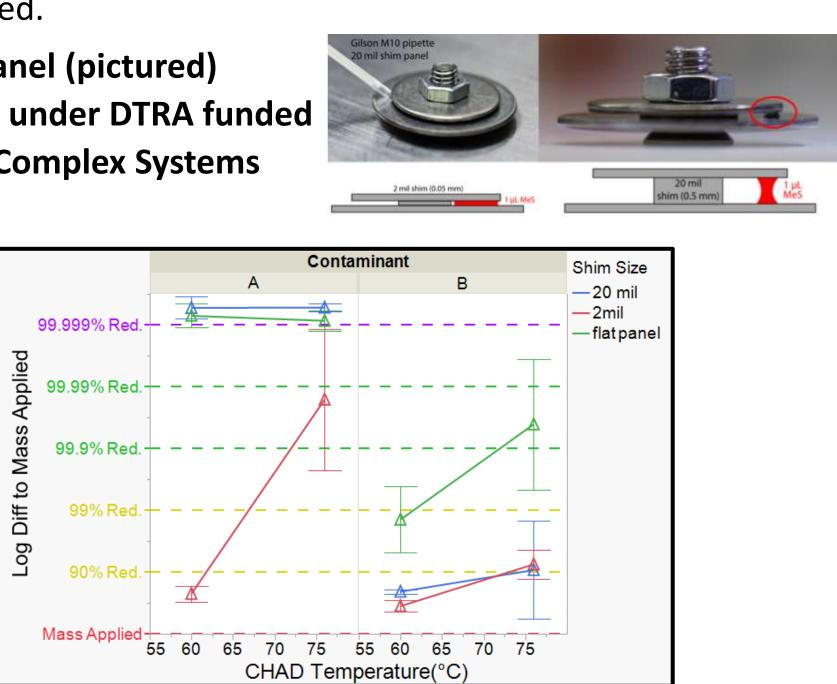
A 4 h treatment of Shim panels showed a substantial degree of contaminant removal for A at both 76°C and 60°C temperatures. The different temperatures produced a different result only for the small Shim size (2 mil). For B, higher temperature produced more removal for all tested materials including the flat panel.
