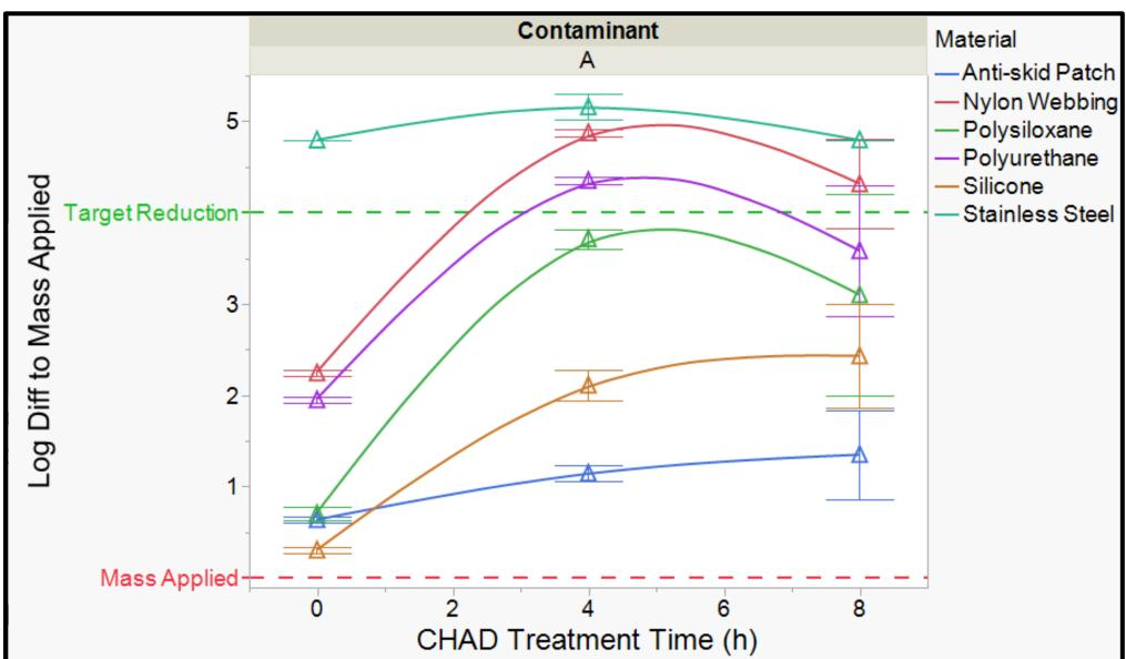
For contaminant A, weathering (treatment time = 0) reduced the contaminant by >1 log for 3/6 of the materials (Nylon, Polyurethane, and Stainless). Silicone, Anti-skid and Polysiloxane retained most of the contamination through the 24 h aging time. 4 h of CHAD treatment removed a significant amount of contaminant, achieving the 4-log target reduction for Polyurethane and Nylon. Additional treatment time increased the removal of the contaminant as well as variability across the replicates.
